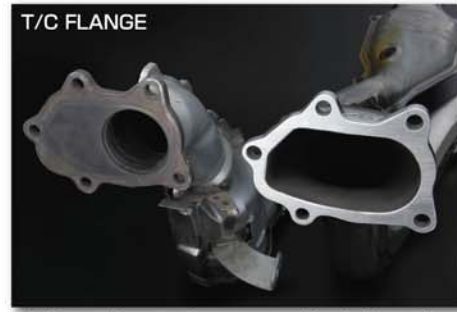
Significant diameter increase resulting in dramatic exhaust flow improvement.
